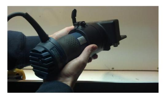
b. With the motor raised up and the power switched off, make a dry run on the ski to insure there are no obstructions and to practice the motion used when grinding.
